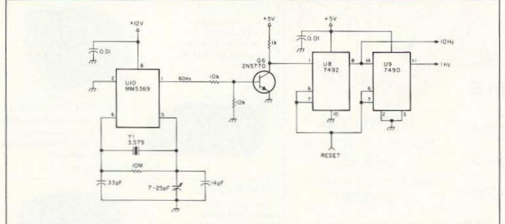
Figure 1. The Heath IM-2410 timebase frequency is generated by an adjustable 3.579 MHz. crystal oscillator/divider, U10.
